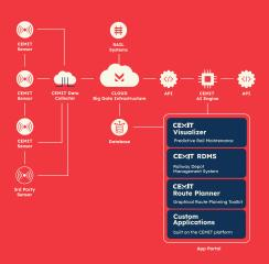
Unlike other intelligent condition monitoring systems, CEMIT has chosen the concept of low-cost and high data volume. Our system can integrate various data sources. This could be open-source data, for instance weather data or other types of environmental data, and it could be siloed data held by the rail operators, for instance sensor data from on-board sensors in trains, or stationary sensors deployed across the rail infrastructure, or information about how much load each train is carrying.
