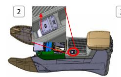
1-2. Chock the wheels and pull the switch to set the parking brake. OPT
