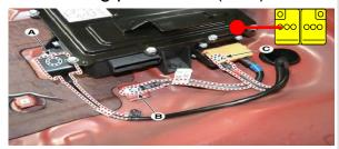
1. After disconnecting (-), (+) terminal of 12V battery, disconnect the low voltage battery cable(A), ground cable(B), inverter power cable(C) in serial order.
