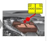
3. Battery in the motor compartment
