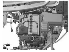
3. Battery in the engine compartment
