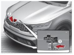
2. Raise the hood slightly, push the secondary latch up (1) inside of the hood center and lift the hood (2)
