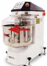
After the machine has been connected to the electrical supply, first of all check the direction of rotation of the kneading spiral and the bowl. Seen from above, both kneading spiral and bowl should rotate clockwise. The arrow on the bowl indicates the rotating direction of the bowl.
