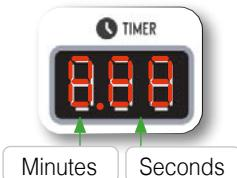
The timer for the first and second cycle is located at the upper side of the panel. The timer indicates the mixing time in minutes and seconds. The timer is set by means of the **+** and **-** keys. If you press the **+** the set time will increase. The maximum time that can be set is 10 minutes. Press the **-** key for reducing the set time.
