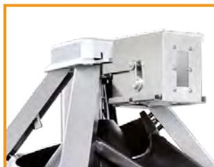
Before reaching the output, the dough will pass the flour dispenser. This can be set to dispense more or less flour by means of the plates at the bottom. After passing this, the dough reaches the output (C).
