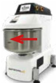
After the machine has been connected to the electrical supply, first of all check the direction of rotation of the kneading spiral and the bowl. Seen from above, both kneading spiral and bowl should rotate clockwise. The arrow on the bowl indicates the rotating direction of the bowl.
