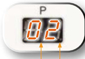
Press the program button to save the program. The two dots will turn off.
