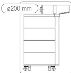
It is recommended that to mount a hood with extractor fan directly over the oven to discharge steam and cooking smoke out of room, Ø200 metal bellows is needed to connect the hood with opening on the wall or roof, thus the risk of corrosion and short circuit caused by moisture can be reduced to the greatest extent.
