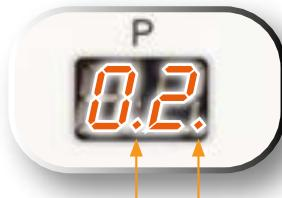
Hold down the program button for 5 seconds until the two dots start flashing. Use the or to select the program number you want to set (e.g., 2).
