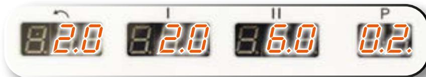
Set the timers for reverse direction, first and second gear.
